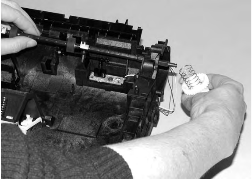
Figure 78. Removing the paper-feed roller (5 of 5)
